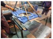
5. Once the body is split 2 parts, the sealing ring will be removed and new seat will be installed. It is important to hit the sealing ring softly but uniformly to avoid damaging it
