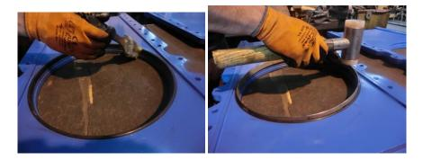
7. We will also change if necessary the 2 body carboard gaskets
