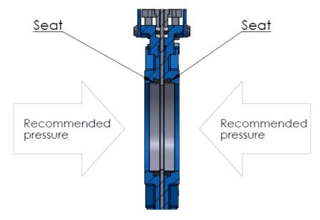
\*Note that the direction of fluid need not always be equal to the direction of pressure.
