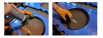
6. After the new seat is installed, the old or new sealing ring will be replaced. Grease (non hydrocarbon based) will help in this process. Please hammer the ring with care.
