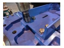
3. Likewise, shaft & knife nuts will be loosened, removing the complete actuator.
