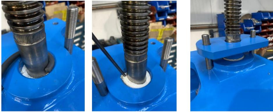
6. Install the original gland follower tightening the nuts progressively. Check that the distance between the gland follower and shaft is equal in all areas. Finally install the support plate.
