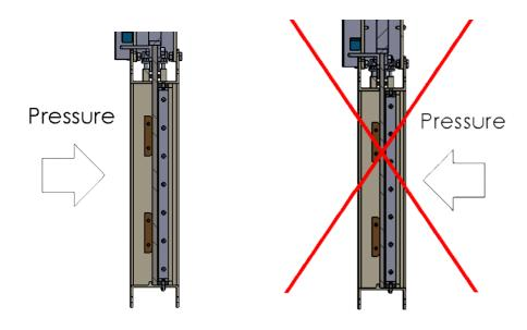
Depending on the drive, and providing the installation so permits, the valves may be assembled vertically, horizontally and even upside down, although we recommend that they be installed vertically.
